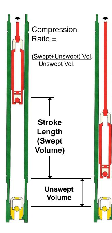
High Compression Ratio Helps Prevent Gas Lock But, Space Pump High or High Tubing Pressure and Gas Lock Possible
