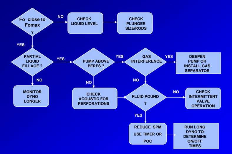
Note: Fo from Fluid Level and Fo from Pump Card should be near FoMax
